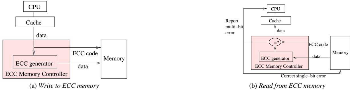
Figure 1: Read/Write Operations for ECC Memory
